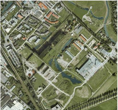
Fig. 12. Orthographic photo showing EVA-Lanxmeer during construction. Note the lakes, the forest strip, the intimate gardens in top and the constructed wetland immediately next to the big building to the East. Elevation 1 km  $\odot$  Google Earth
