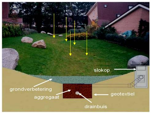
Fig. 26. Conceptual section of wadi at Ruwenbos, Enschede. Depression, filter substrate, infiltration box, drain pipe, geo textile and overflow structure (from Palsmaa, 2008)
